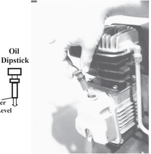
Figure 1. Checking the Oil Level
